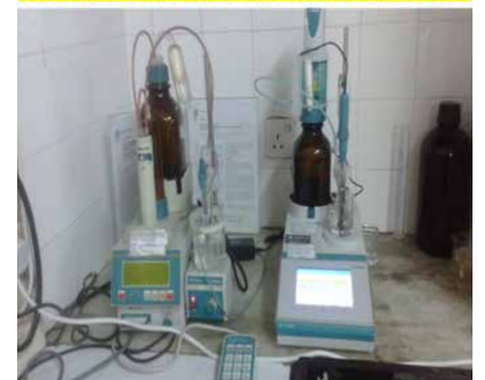
Base Number Test: TBN Method: ASTM D2896
