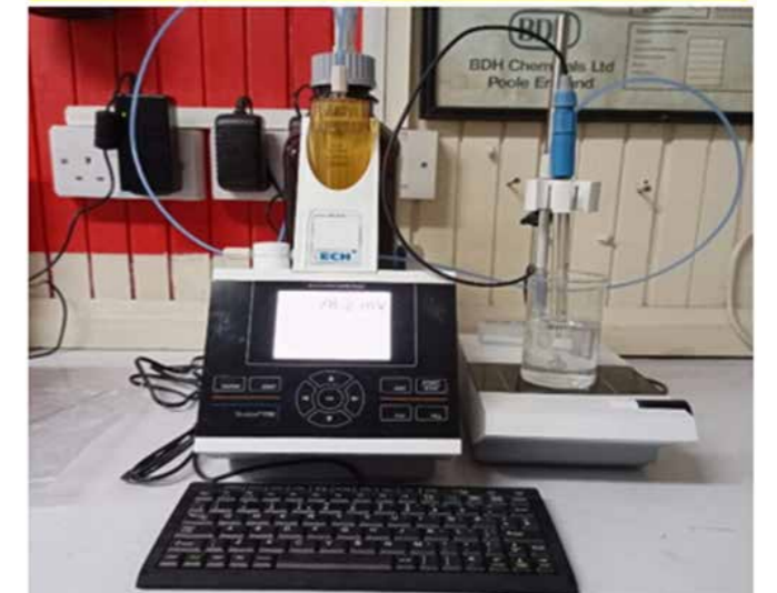
Acid Number Test: TAN Method: ASTM D664
